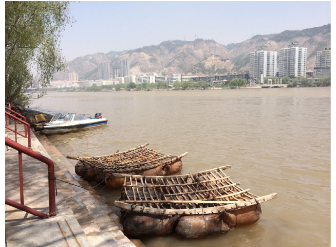
Sheepskin rafts are an ancient means of transportation in northwestern China. Sheepskins are sewn, sealed, inflated, and then fixed with a rope onto sticks.
